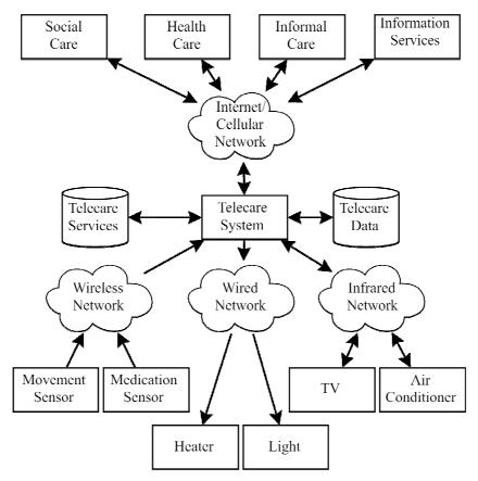
Figure 1. Example MATCH system environment
