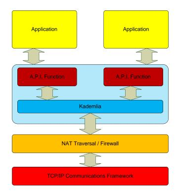
Figure 4.2: System Block Diagram for Bushfire Framework [7] (Adapted)
