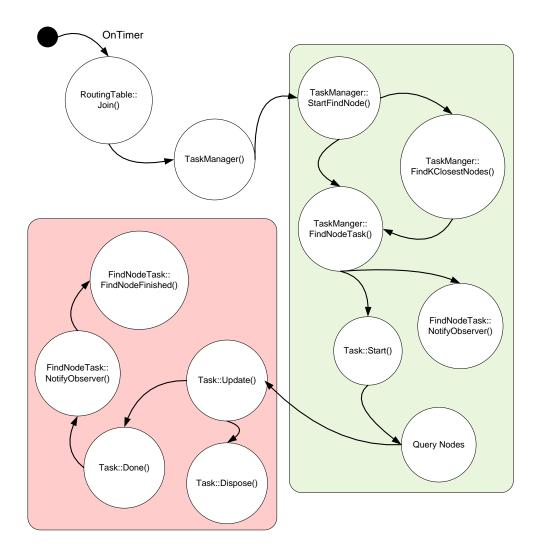
Figure 4.6: Quasi-State Diagram of Overlay Network Join Process
