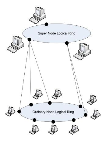
Figure 2.9: Hierarchical (Super Node) Topology Overlay Classification
