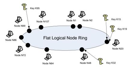
Figure 3.5: P2P Address Space: 1 Dimensional (Flat), Logical Ring [7] (Adapted)
