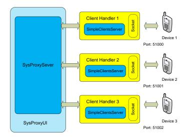
Figure 4.10: System Block Diagram of SysProxy
