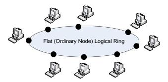
Figure 2.8: Logical Ring of Nodes illustrating a Flat Topology Overlay Classification
