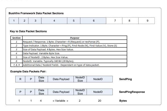
Figure 4.4: Example of Bushfire Framework Data Packet Construction Design
