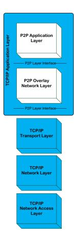
Figure 2.3: A P2P System Layer Diagram
