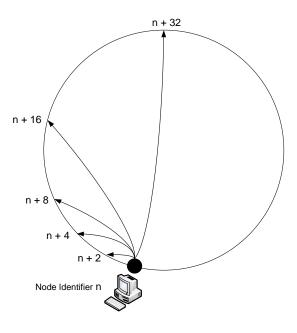
Figure 3.2: Chord Overlay Routing Design
