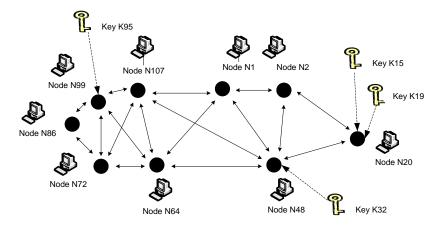
Figure 3.6: P2P Address Space: Mesh Topology [100] (Adapted)
